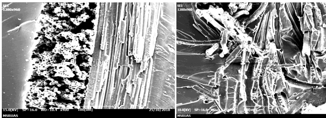
Fig. 9 Shows tensile fracture of hybrid composites using carbon-jute and carbon-hemp
