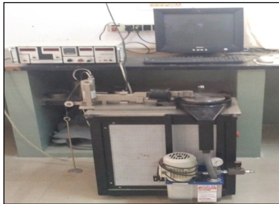
Fig. 1. Schematic view of pin-on-disc dry sliding wear test machine.
