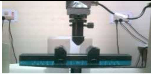
Fig 3 Flexural test in Universal Testing Machine
