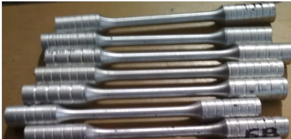
Figure: 4 Prepared Tensile specimens as per ASTM E8 standard.
