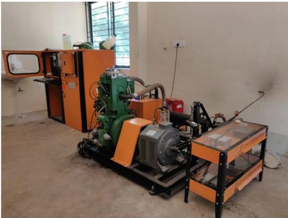
Figure 2: Photograph of Diesel engine test rig
