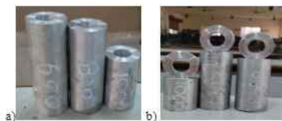
FIGURE 5.a) Casted specimens b) Samples machined from cast
