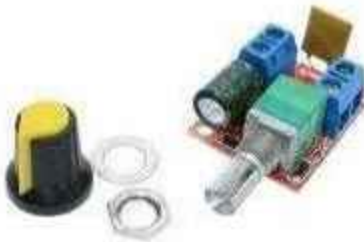
FIGURE 5: Speed Controller Switch
