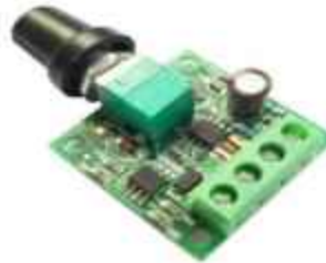
FIGURE 6. .Speed controlling unit
