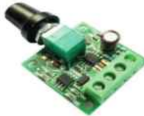
FIGURE 6. .Speed controlling unit
