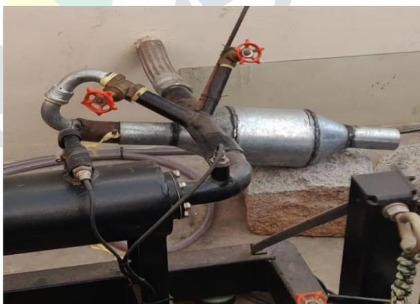
**Figure 10** Diesel engine exhaust having Catalytic converter only
