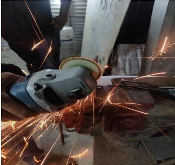
**Figure 3** Cutting of sheet metal
