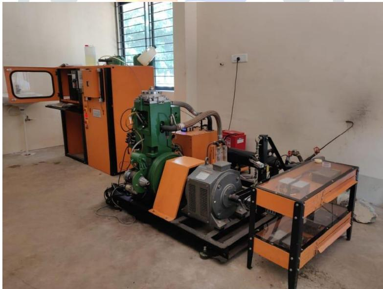
**Figure 5.**Diesel engine test rig
