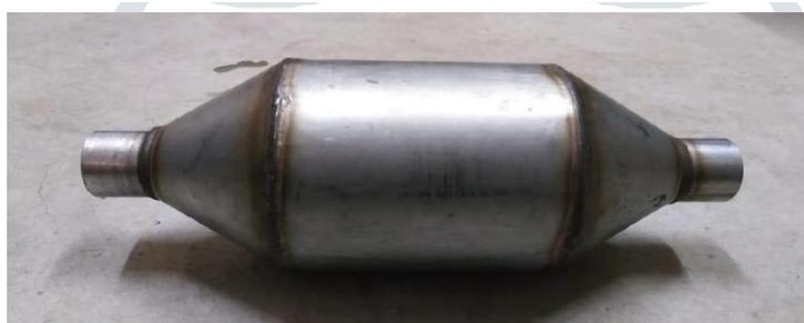
**Figure 6** Diesel Particulate Filters
