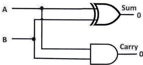
Figure 1: Half Adder circuit
