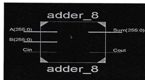
Figure 1: RTL View of RCA
