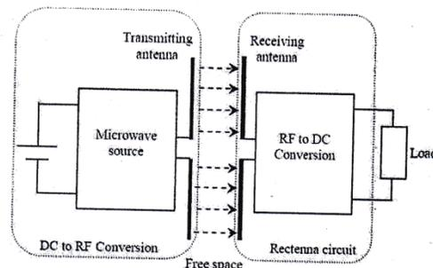
Fig.1 basic design of wireless power transmission
