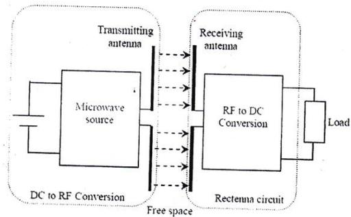
Fig.1 basic design of wireless power transmission (Image courtesy form reference8)
