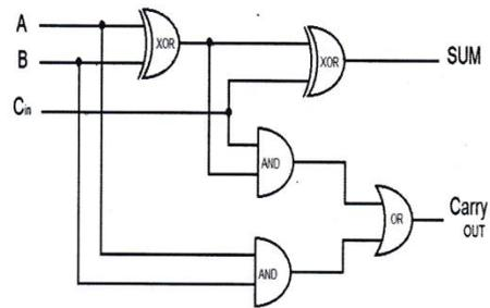
Figure 2: Full adder circuit
