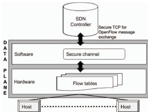
Fig. 2. OpenFlow communication between SDN switch and controller
