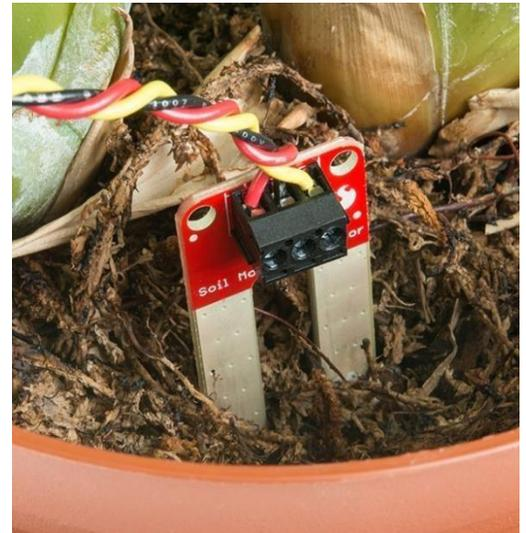
FIGURE 1. Soil moisture sensor
