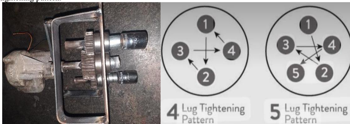
FIGURE 1: Multi-nut lightener and lug tightening pattern
