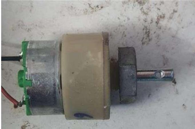
**FIGURE 2. DC Electric motor**
