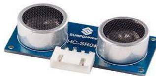
**FIGURE 2:** Ultrasonic sensor
